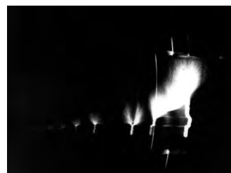
Triggering picture of a SRAT with a rotative high speed camera.
